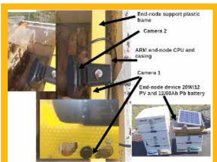
Slika 4. Sustav kamera za praćenje grinje V. destructor (izvor: https://www.mdpi.com/signals/signals-03-00030/article_deploy/html/images/signals-03-00030-g001.png )
