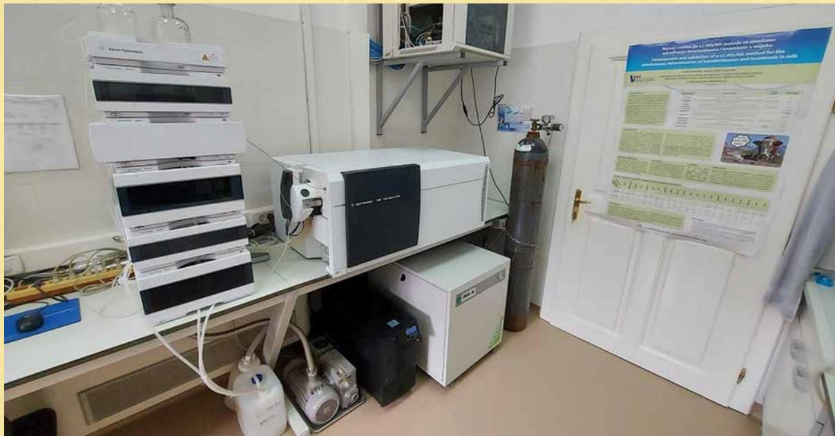
SLIKA 1. VEZANI SUSTAV TEKUĆINSKE KROMATOGRAFIJE – TANDEMNE SPEKTROMETRIJE MASA (LC-MS/MS)
