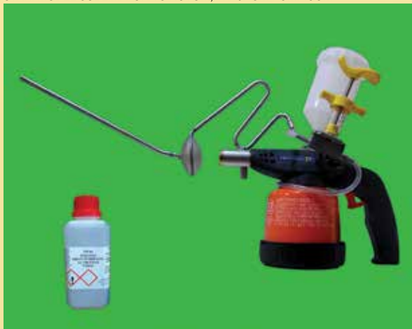
STARI MODEL SUBLIMATORA S NOVOM, TRAJNOM PUMPICOM
