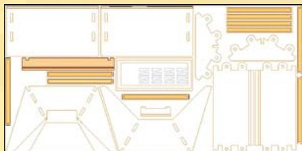
NACRT COLORADO TOP BAR (VERZIJA 3.0) - ZA IZRADU COLORADO TOP BAR KOŠNICE BILA JE POTREBNA 1 ŠPERPLOČA, CNC GLODALICA SA ČELIĆNIM RAČUNALNO NAVOĐENIM SVRDLOM, DATOTEKA S NACRTOM.
